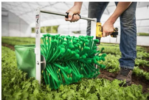
**Figure 1** Quick cut greens harvester.
